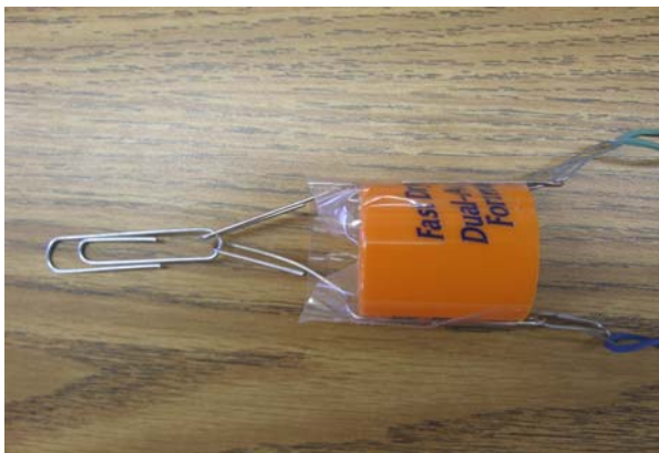
Figure E8 – Cup that holds atom prior to shooting.
