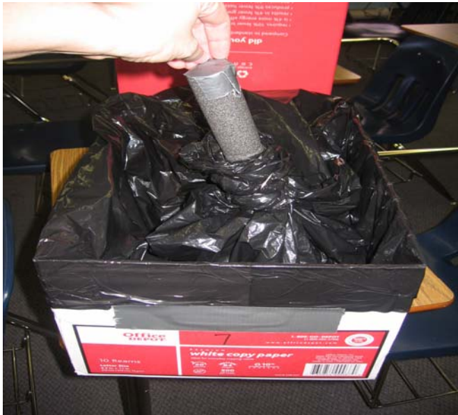
Figure E4 – Atomic Force Macroscope showing probe and black garbage bag covering the box.
