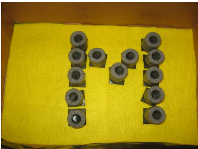
Figure E5 – Bottom of paper box (Atomic Force Macroscope) showing the design pattern attached to the felt.
